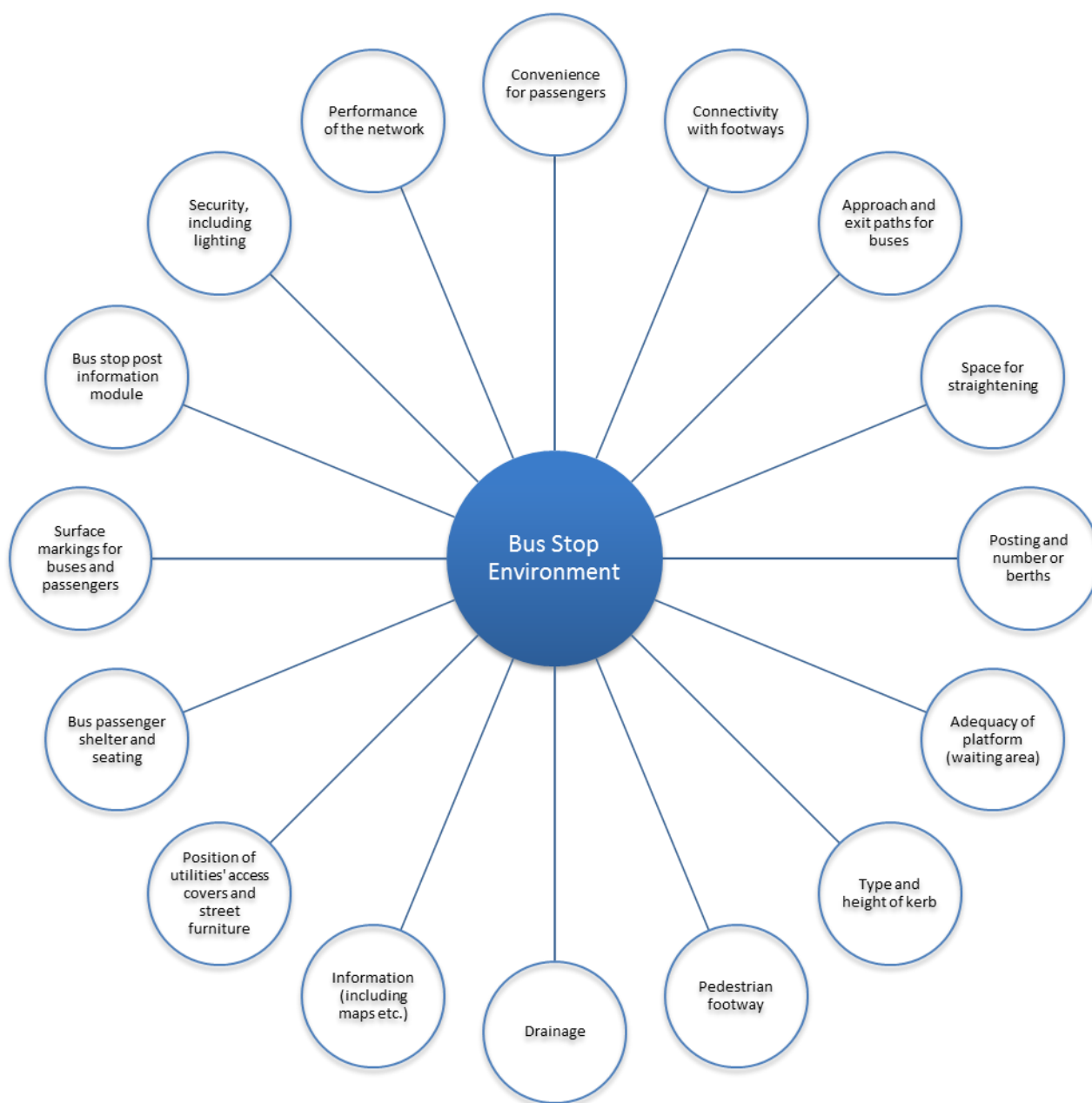
Figure 3.2: Issues to Consider at Bus Stops (Adapted from Transport for London Accessible Bus Stops)
