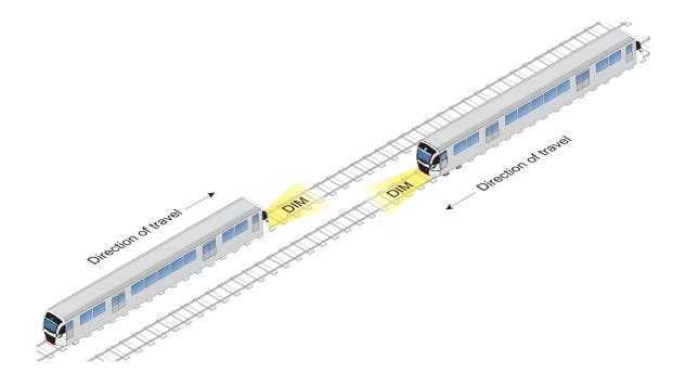
FIGURE: 3.3: When approaching and crossing the lead end of opposing Rail Traffic.
